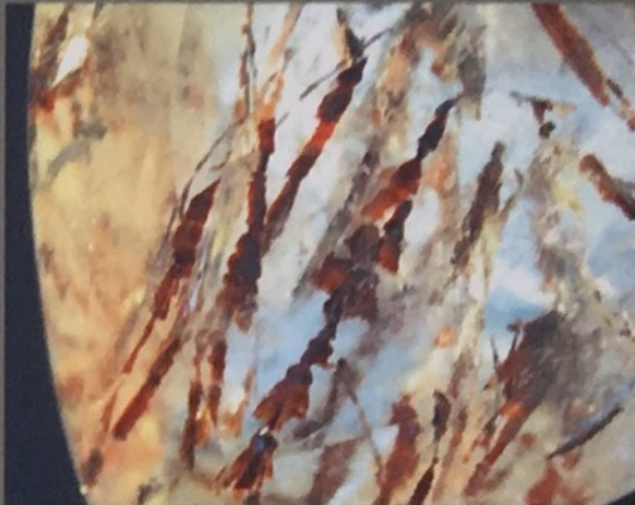
Image | Iron oxide 'beetle leg' inclusions in strawberry quartz
