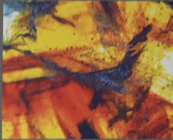
Image | Colour zoning in sphalerite with fractures, and unknown primary inclusions
