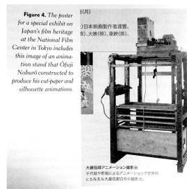
The animation stand is perhaps the most central technology in animation. A rack with several glass planes with a camera mounted on top. images or objects are placed on the glass layers, the camera composite the various image elements together into one image. This layer structure reoccurs in many modern digital softwares for image and animation.
